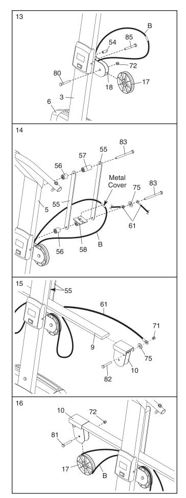
17. Hold a Large Pulley (17) inside the upper cable (B). Attach the Pulley to a Pulley Bracket (10) with an M12 x 58mm Button Bolt (81) and an M12 Nylon Locknut (72). Make sure that the cable is routed as shown in the CABLE DIAGRAM on page 18.
